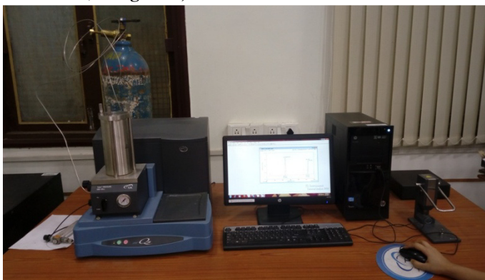
Pressure Differential Scanning Calorimeter (Q20) model Q20 from TA Instruments in Centre of Materials Science.
